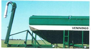
Two electric actuators operate seed and super doors by a hand held control box with a 14' 6" (4500mm) reach. Hydraulic operated rams open and shut cut off doors inside of both super and urea bins which are again operated from the same
