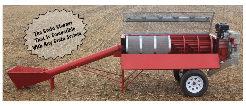
The GT Grain cleaner is completely portable on 185/60R 14" wheels. It is versatile and flexible so that you can insert it into about any point of your grain handling and storage system. The chain driven drum gently yet thoroughly removing fines, chaff, weed seeds and other foreign material.
