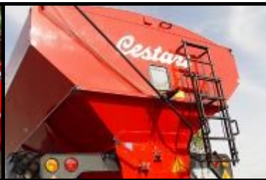
External & Internal Ladders. Rear ladder folds up keeping it well out of the way when not in use
