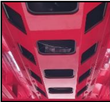
Large trapdoor fitted to the bottom of bin with quick and easy cleanout of bin
