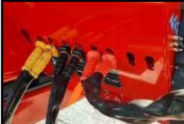
Organiser for hoses and light cables. One pair of the hoses for the hydraulic folding auger & the other pair for shut of covers for floor auger
