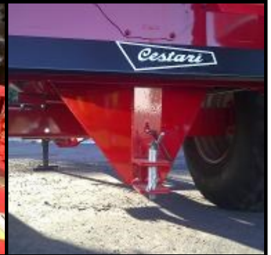
Tow hitch fitted to the rear of the bin for towing augers or portable bins for on farm use only (check legal requirements in your state)
