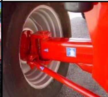
Front steering axle made from 16mm Folded Plate 230mm x 160mm heavy duty bearings and 10 stud hubs
