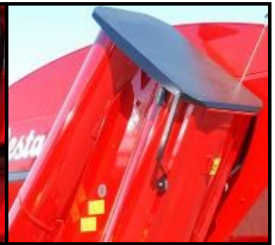
Join in auger is covered when auger is folded
