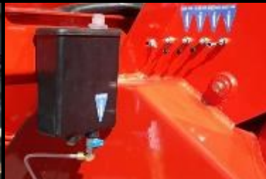
External centralized lubrication point makes lubrication and maintain a simple task
