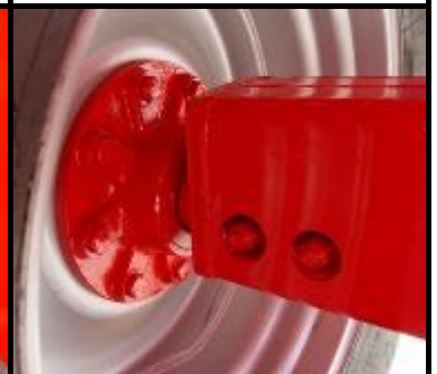
Rear axle made from 13mm Folded Plate 320mm x 160mm heavy duty bearings and 10 stud hubs
