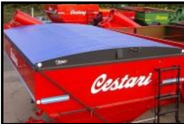
Heavy Duty Roll over Tarp fitted to bin
