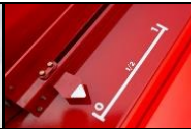
Indicator on front of bin shows position of shut off doors allowing bin to be unloaded at any speed
