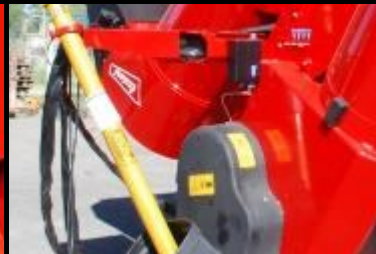
Pivoting PTO and hose holder fitted to front of bin
