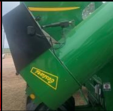
Adjustable discharge spout simply adjust the direction of grain flow by pressing a toggle switch
