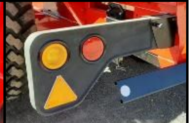
Tail Stop and turn indicators on folding arms
