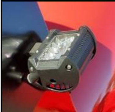
Led Work light fitted to discharge auger
