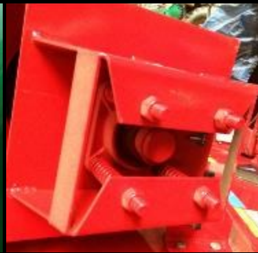
Discharge auger is fitted with spring led top bearing in case auger is folded out and flighting is not in correct position
