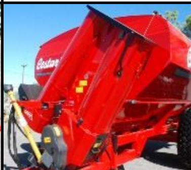
31,000 Litre bin takes 3.5 minutes to unload 43,000 Litre bin takes 4 minutes to unload
