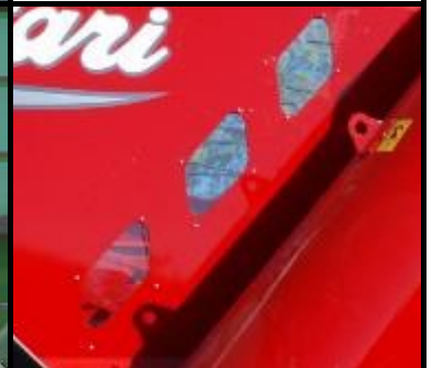
Three large viewing windows fitted to the front of the bin
